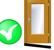
If on the other hand it slants <u>heavily downward</u> away from the hinged edge of the door leaf, you should consider using a brush door sweep instead of the WAVE door sweep.
