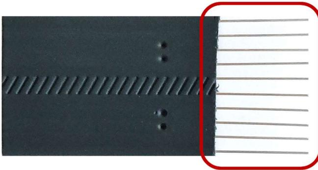
The rodent proofing barrier consisting of 10 solid wires of stainless steel with a diameter of 1/25 in (1 mm) stripped from the thermoplastic vulcanizate. The spacing between the wires is 1/5 in (5 mm) – too little for a mouse to squeeze through.
